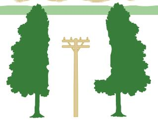
Although cutting from ground to sky is preferred, trees can be trimmed in a side cut or an L-shaped cut to ensure their health and sustainability while keeping branches a safe distance from power lines.
