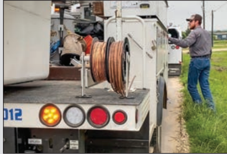
Apprentice lineman Taylor Rutledge performs a walk-around inspection of his truck to check for potential backing hazards, loose straps, low tires or other problems. Sarah Beal photo
