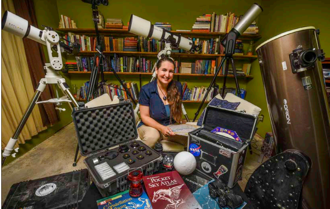
Dawn Davies writes online reports about night-sky viewing, focusing on state parks. Her tools include a variety of telescopes, binoculars, lens adapters, charts and books. The 80mm white telescope on the left is ideal for deep-sky viewing; the large copper telescope at right uses mirrors instead of lenses. Photos by Sarah Beal
