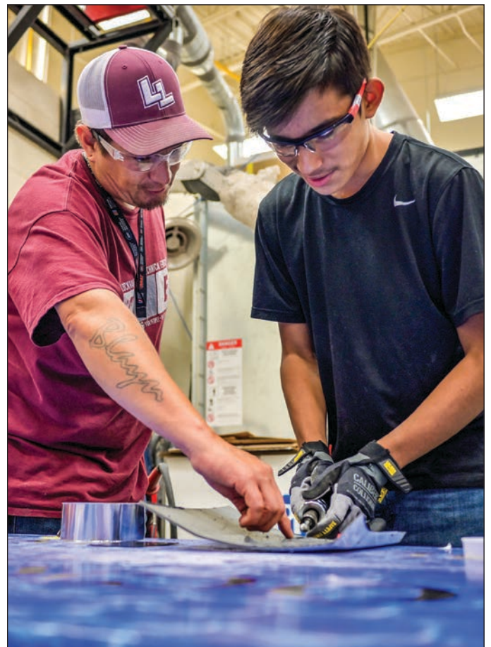
Lockhart High School collision repair student Blayn Hernandez, right, gets directions on the intricate process of repairing a plastic bumper piece from his teacher and father, AJ Hernandez. The skill and precision it takes to use the high-tech plastic welding tool is necessary for career certification.
