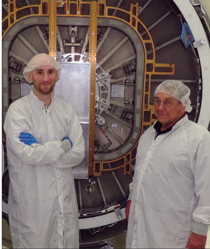
Tyler Holden, left, and Quad-M founder Victor Dube in 2018 in Dulles, Va., at the Orbital ATK facility. They were checking the fit of their first Slingshot bracket, the golden structure behind them, on the front of the Cygnus spacecraft. The Slingshot, built by Quad-M, is used to deploy cube satellites into orbit. Orbital ATK, which produced the Cygnus spacecraft, was later purchased by Northrop Grumman.
